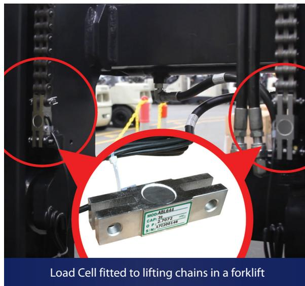
Load Cell fitted to lifting chains in a forklift
