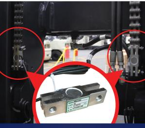
Load Cell fitted to lifting chains in a forklift
