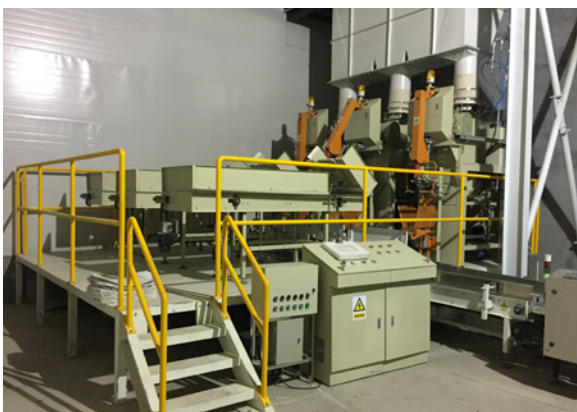
Automatically picks up and hangs various bags on your weigh scale system.
