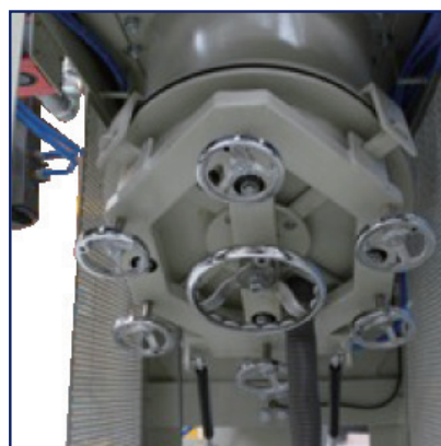
Rear Cleaning Hatch
