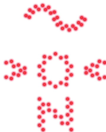
Annunciators for center of zero (middle), motion flag (top) and net (bottom)
