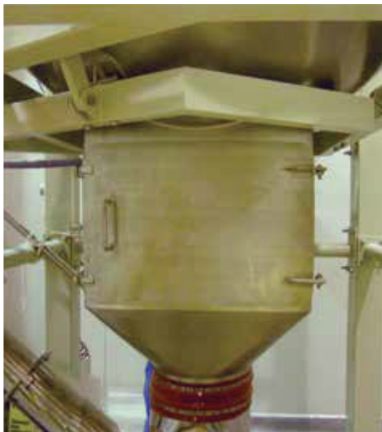
Bag Untie Access Door For Bulk Bag Emptying System
