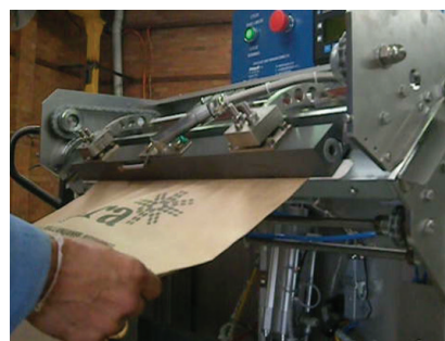
Sealing Process (Covers removed for Demonstration)
