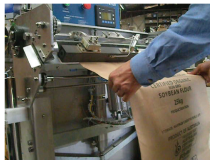
Sealing Process (Covers removed for Demonstration)
